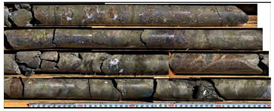
Photograph of G11-468-03 from 256.45m to 258.50m (2.05m) grading 40.8% Zn+Pb (30.5% Zn and 10.3% Pb) and 384.7 g/t Ag, Ballywire Prospect, Ireland
