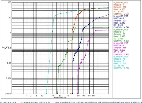
Figure 14.13 Composite BaSO<sub>4</sub>% - Log probability plot overlays of mineralisation per MINZON
