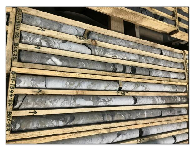
Figure 12.1Drillhole G11-1344-02: Core trays showing interval ~64.8 to ~70.5 m, with mineralogical<br/>assemblage consisting of pyrite, sphalerite and minor galena
