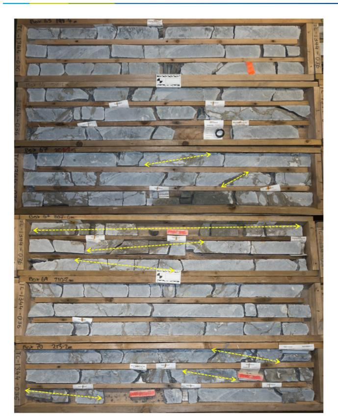
Figure 9.1 Picture of core from drillhole TC-1344-036, showing steep component to Mineralisation likely to be fractal on a larger scale (Photo courtesy of John Kelly SLR Consulting, February, 2017). Drill core is NQ in size.
