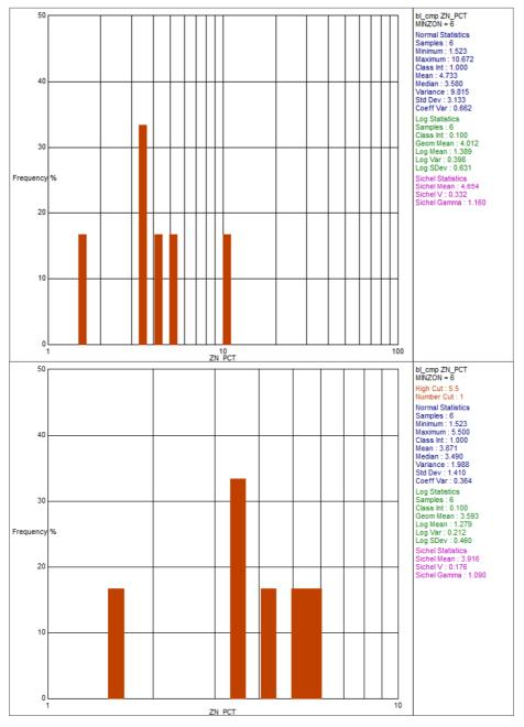
**Figure 14.14** Zn% (MINZON = 6) - Log Histogram Plots Uncut (top) and Top-Cut (bottom) (Source: CSA Global, 2018)
