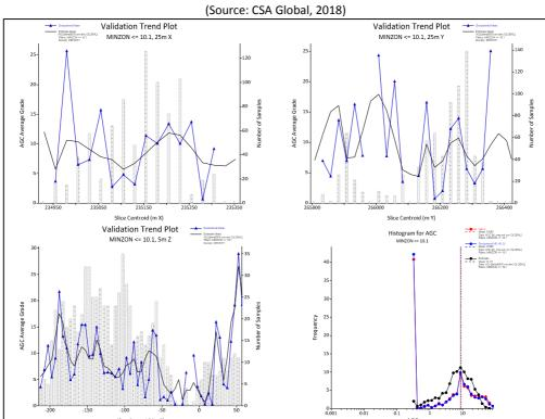
Figure 14.29 Ag g/t Swath plots and histogram, block model (black) vs. declustered composites (blue) (MINZONs 1-10) (Source: CSA Global, 2018)
