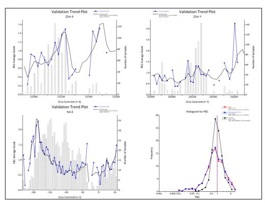
Figure 14.28 Pb% Swath plots and histogram, block model (black) vs. declustered composites (blue) (MINZONs 1-18)
