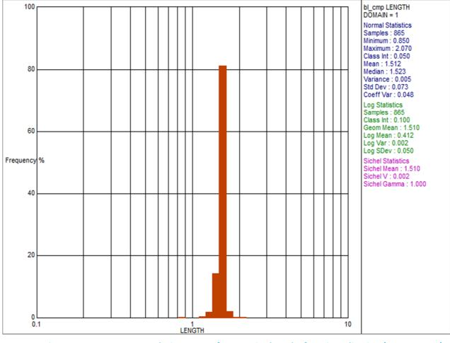
Figure 14.9 Log Normal Histogram of composite lengths for mineralisation (DOMAIN = 1)
