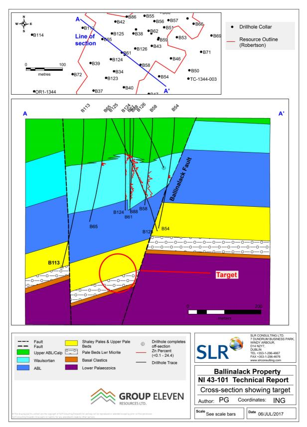
Figure 9.2 Pale Beds target underneath existing shallower prospect within the Waulsortian
