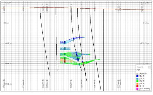
Figure 14.24 Section view – Pb% Grade Model and composites (Source: CSA Global, 2018)
