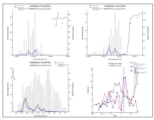
Figure 14.30 BaSO<sub>4</sub>% Swath plots and histogram, block model (black) vs. declustered composites (blue) (MINZONs 1-4, 18) (Source: CSA Global, 2018)
