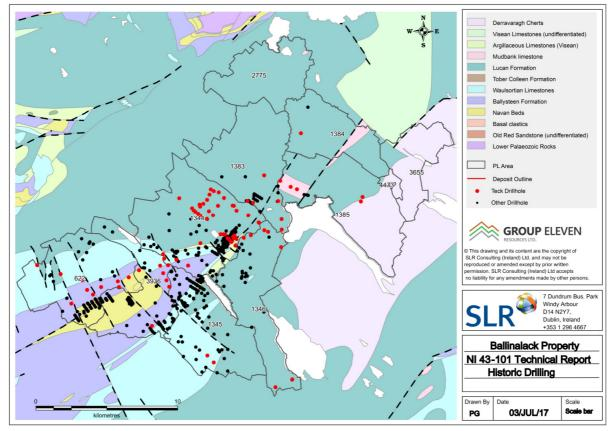
Figure 6.3 Previous drilling on Ballinalack group of PLs.
