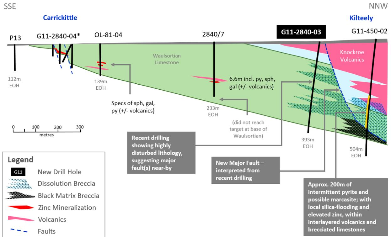
Note: 'sph' = sphalerite (zinc-bearing mineral), 'gal' = galena (lead-bearing mineral); 'py' = pyrite (iron sulphide);
