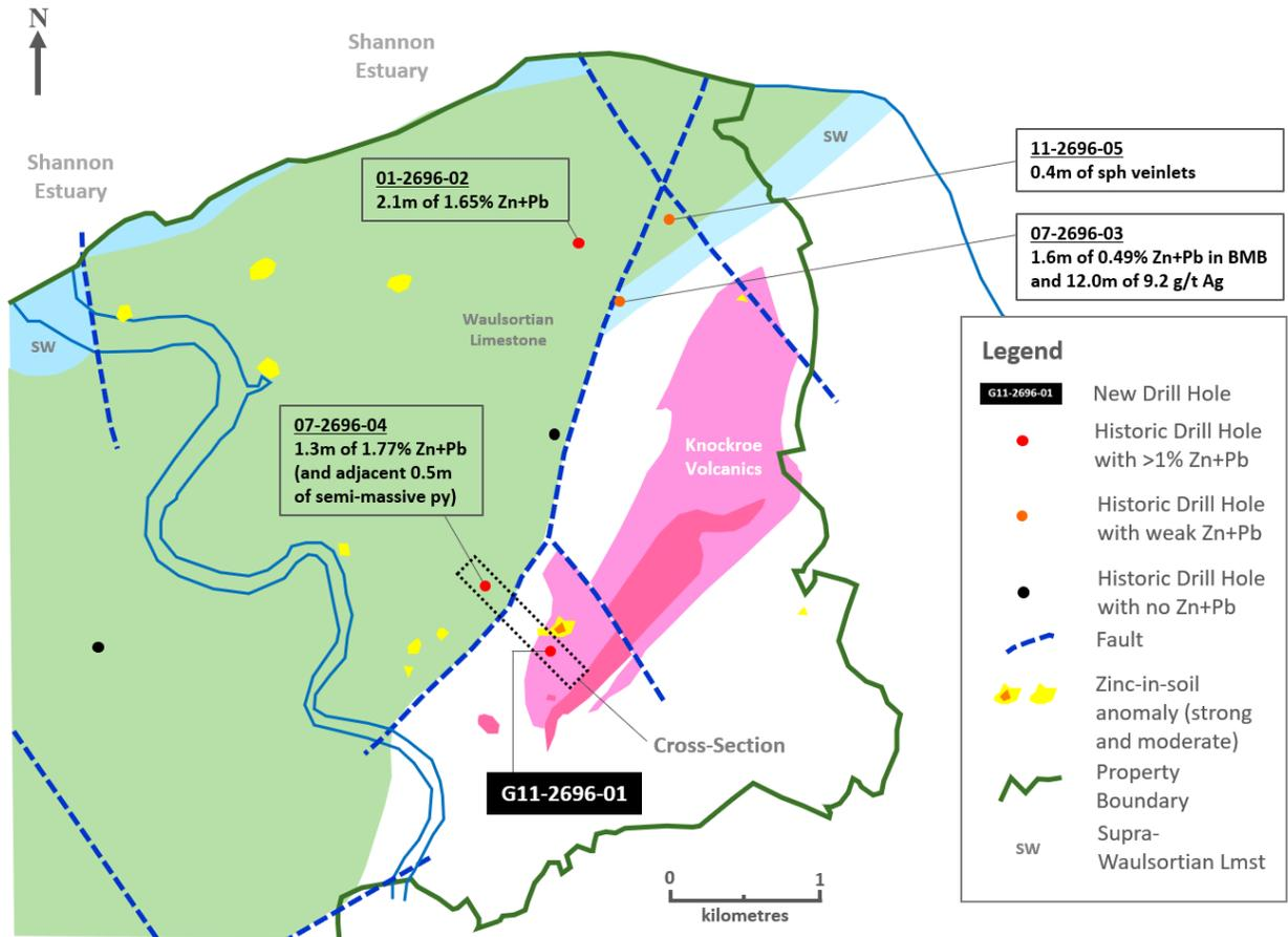
Note: 'Zn' = zinc; 'Pb' = lead, 'sph' = sphalerite (zinc-bearing mineral), 'gal' = galena (lead-bearing mineral), 'py' = pyrite, 'Waulsortian Lmst' = target horizon for zinc in Ireland (limestone), "BMB" = black matrix breccia (prospective for zinc);
